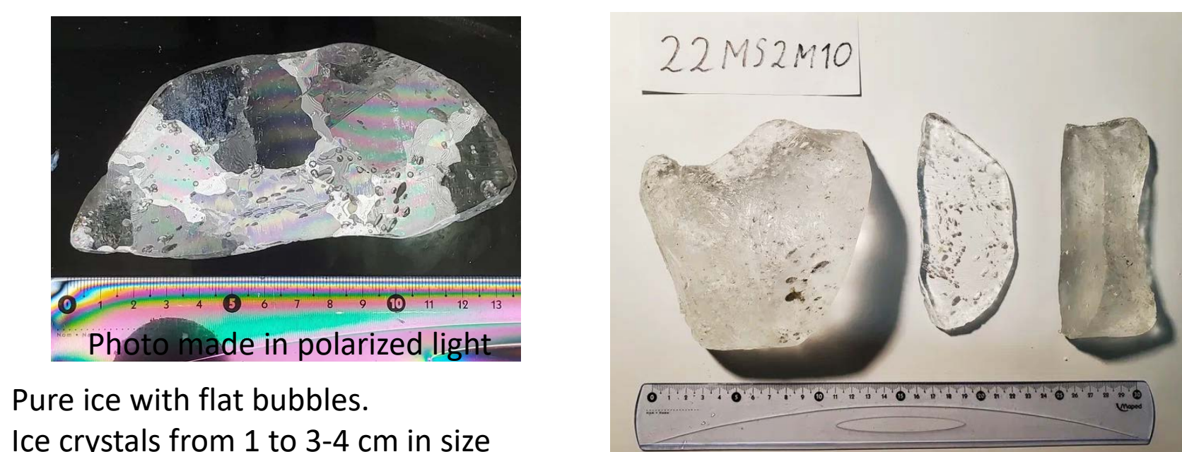
Pure ice with flat oriented bubbles. Large ice crystal more than 10 cm in height
