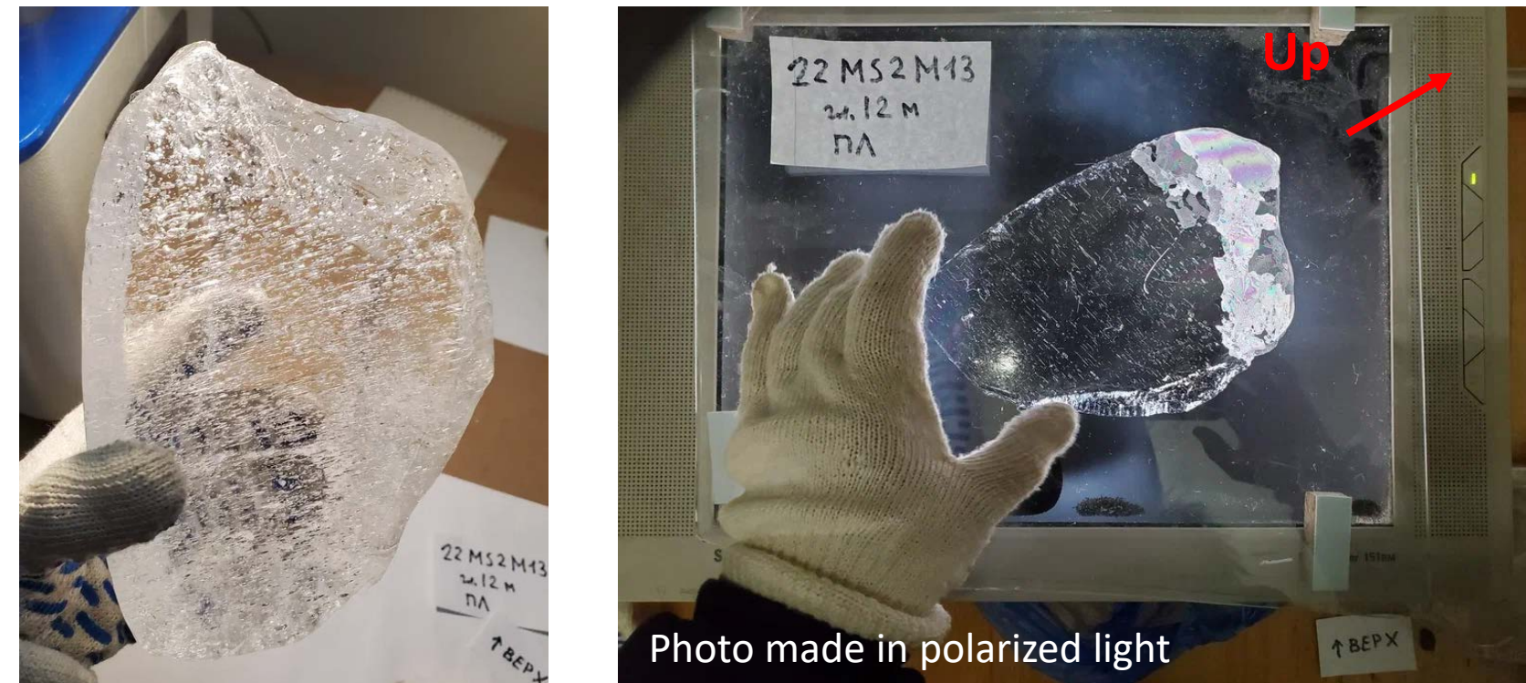
Pure ice with flat oriented bubbles. Large ice crystal more than 10 cm in height
